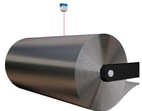
**Measurement of coil diameters**
