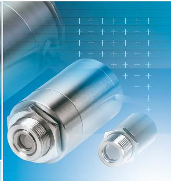
Infrared pyrometers determine the object temperature without contact based on the infrared radiation emitted by the object according to the radiation law of Planck and Boltzmann. A detector converts the incoming infrared radiation into an electrical signal. An amplified and linearized temperature value can then be used for further processing. The use of infrared pyrometers opens up various opportunities to measure and display temperature profiles in numerous fields of applications.
