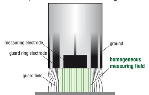
Common capacitive sensor (coaxial)
