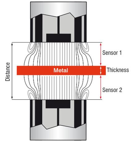
$$\text{Thickness} = \text{Distance} - (\text{Sensor 1} + \text{Sensor 2})$$
