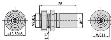
Max. leak rate  $1 \times 10^{-9}$  mbar · l s<sup>-1</sup>, compatible with connector type B
