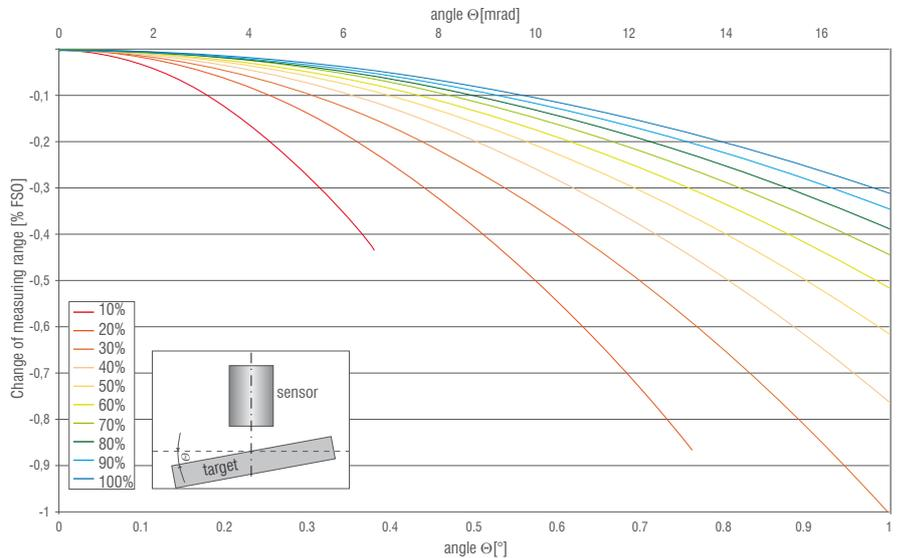
**Example illustration of the influence using the CS02 sensor as an example, consideration of a tilt angle of max. 1° for different sensor distances.**
