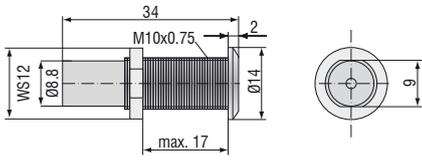
Max. leak rate  $1 \times 10^{-7}$  mbar · l s<sup>-1</sup>, compatible with connector type B
