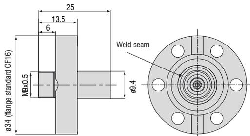
Max. leak rate  $1 \times 10^{-9}$  mbar · l s<sup>-1</sup>, compatible with connector type B
