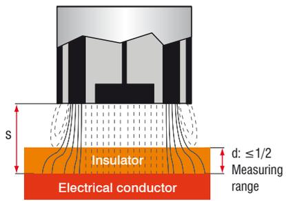
**Thickness measurement of insulators**
