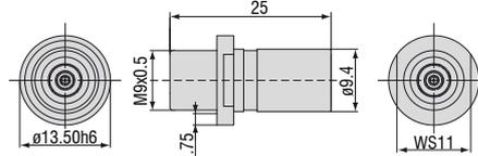
Max. leak rate  $1 \times 10^{-9}$  mbar · l s<sup>-1</sup>, compatible with connector type B
