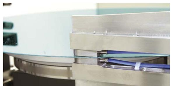
Wafer thickness measurement with two capacitive sensors
