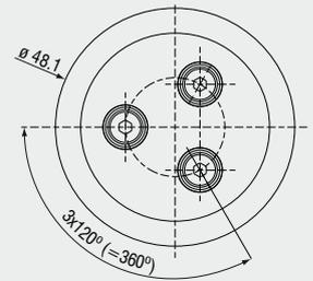
Bore hole for fixing screws  $\varnothing$  20mm
