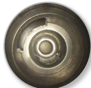
Checking brake cylinder for burrs
