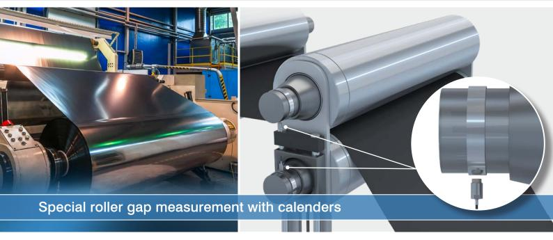
Plastic films, such as electrode films for lithium-ion batteries, are produced using calendering technology. The plastic is brought to the desired thickness between two adjustable rollers. For automatic gap control combined with integrated inline thickness measurement, the nip between the rollers is continuously measured. This task is performed by inductive sensors based on eddy current technology from Micro-Epsilon.
