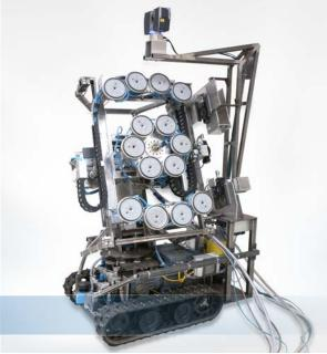
The Institute for Technology and Management in Construction at KIT has developed the climbing robot "MANOLA", which is intended to be used for dismantling contaminated buildings. The robot will climb up facades, detect contaminated areas using a detector and remove them layer by layer. In order not to hit any obstacles and damage the sensitive detector, two additional laser profile scanners from Micro-Epsilon were integrated.
