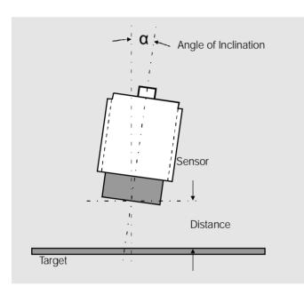
A permanent tilt angle can already be lodged at the Controller with the 3-point linearization. This avoids an influence of this tilt angle to the signal.
