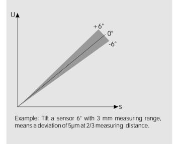
Tilt angles, the controller not linearized for, cause deviations of the measured values in comparison to right angled measurements.
