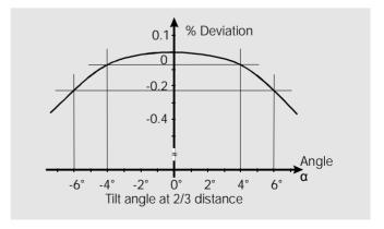
A tilt angle of more than 6 degree is rather possible with unshielded sensors than with shielded, but should be avoided. In principle, only a special linearized sensor provides a precise signal.
