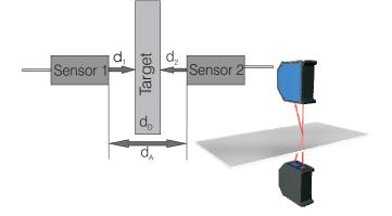
Two sensors are placed at a known distance  $d_A$  on both sides of the measuring object (= target) which each measure the distance to the object. The distances  $d_1$  and  $d_2$  are subtracted from the sensor distance  $d_A$  in order to determine the thickness  $d_D$  of the target.
