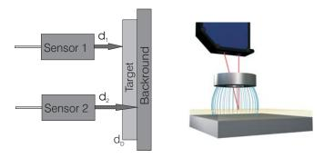
Two sensors are placed at the same distance  $d_1$  from the measuring object on one side of the target. One sensor measures the distance  $d_2$  to the background which is on the opposite side of the object. The thickness  $d_p$  of the target is calculated by
