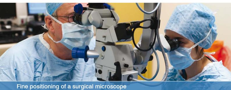
Surgical procedures require a perfect view of the operating area. Here, the surgeon is often supported by a surgical microscope. To enable the surgeon to best position the microscope and to give the surgical team more room to move, the microscope optics are mounted to long arms
