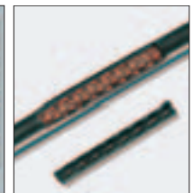
Disbonded cable coating
