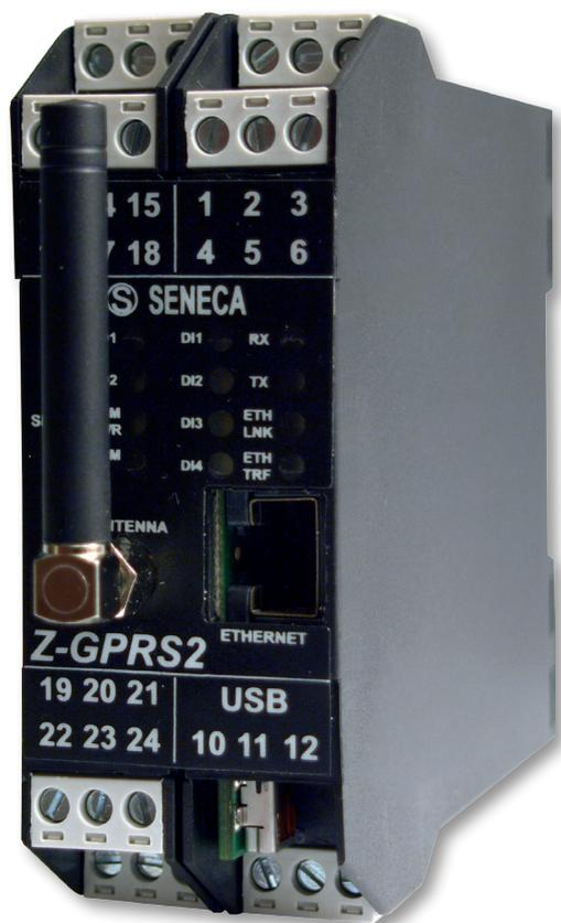
**ALIMENTAZIONE:** 11..40 Vdc; 12..28 Vac (50-60 Hz)
