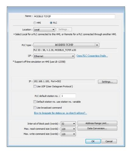
If the client chooses [RS-232] or [RS-485] PLC interface, the [PLC type] must be set to "MODBUS RTU", and its communication parameters also must be configured correctly.
