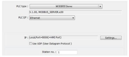
The [Port no.] of MODBUS Server and HMI must be the same. To change the port number, please set in the [System Parameters] » [Model] tab.
