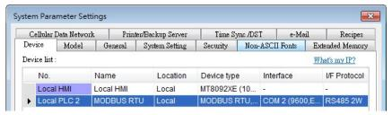
In the setting page of each object, select "MODBUS RTU" in [PLC name], and set the address of MODBUS RTU.
