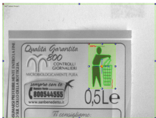
Fig. A 360° Defect Finder Control: Reference Image
