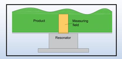
Due to the sensor's distance dependency it is recommended to place the sensor as close as possible to the product, the measured values are available as %H<sub>2</sub>O.
