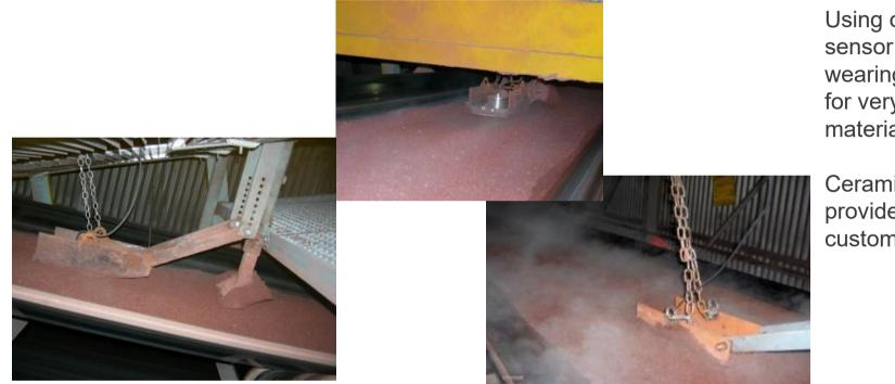
Using of FMS II sensor with 10 mm wearing protection for very abrasive materials !!!
