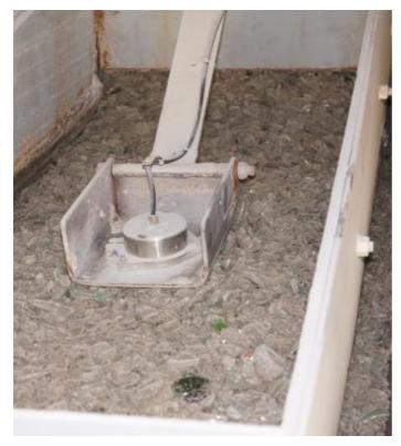
Since then, a further 10 measuring points have been equipped with Litronic-FMSII sensors to ascertain the residual moisture content in quartz sand and recycling glass.
