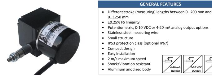
AWP 110 series draw wire sensors; consists of a rotary potentiometer which is controled by stainless steel wire. They make measurement by pulling and rewinding stainless steel wire. Different stroke lengths between 0...200 mm and 0...1250 mm are available. They converts linear motion to potentiometric output.
