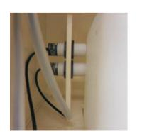
Capacitive proximity sensors belong to a sort of position sensors. Similar to the structure of a capacitor, the probe of sensor acts as one pole of capacitor and another pole is the sensing object. While the sensing object approaches a proximity sensor, the dielectric constant may change between object and sensor. Meanwhile, this causes the circuit to alter.
